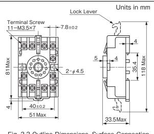
Fig. 3.3 Outline Dimensions, Surface Connection Socket Assembly (11PFA)
