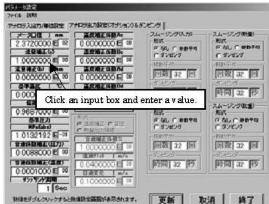
Fig. 8.8.2 Input Procedure for Parameter Settings
