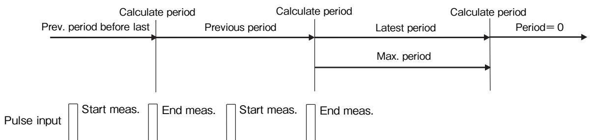
Interpolation – “to read between the lines” - involves a process to run a periodic check for the presence of incoming pulses at intervals of 100 ms; calculate the period based on the elapsed time at the time of check when pulses are missing for a duration beyond the previously measured period of time.
