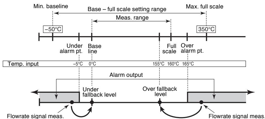
Alarm point and fallback setup range is determined as follows:
