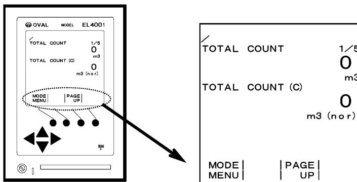
Labels to show functions assigned to function keys in RUN mode (example)
