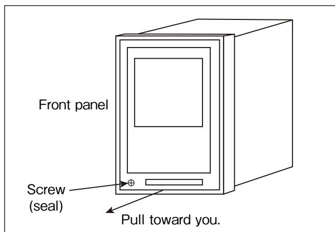
**⚠ CAUTION:** 1. Power must be OFF before you start working with the front panel. Problems do arise if you, with power ON, attempt to gain access to the rear of the front panel.
