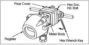
(1) Using the hexagonal wrench key, take off four bolts and separate the meter body and register assembly from the rear cover.
