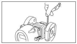
(1) Take off four hex bolts from the meter to separate the register from the meter.
