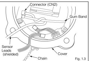
CAUTION: Pulling the connector by wire leads may lead to poor electrical contact at the connector.
