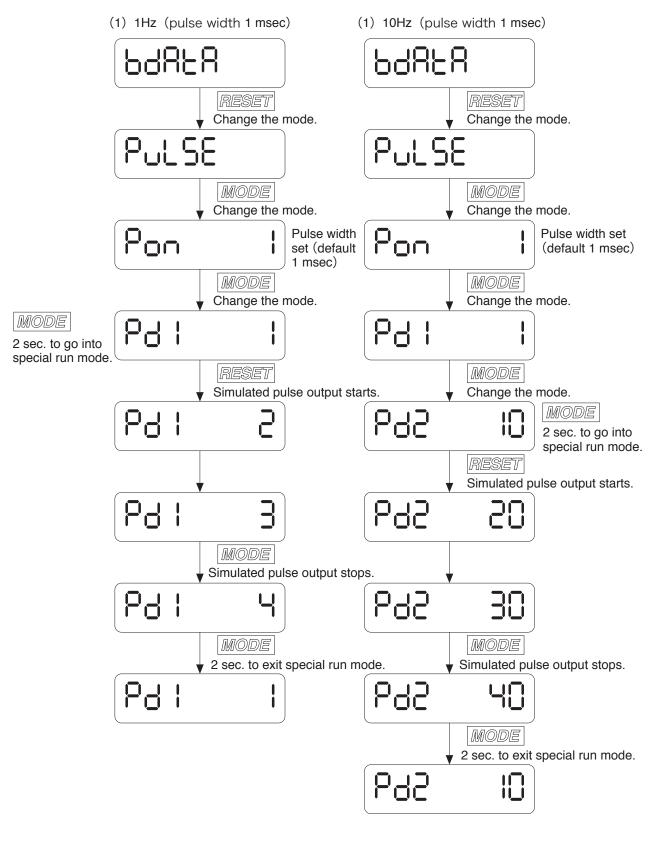
NOTE: In(2)10Hz dummy output above, typical indications are shown.
