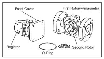
(2) Holding the register and front cover in your hand, separate horizontally. Inspect the measuring chamber and remove scale adhering to components. Exercise care to avoid dropping the rotors or may result in damaging them.
