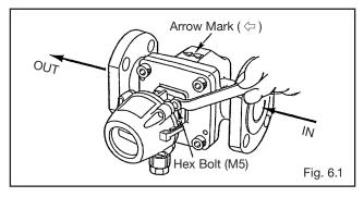
Remove the meter from the pipeline and separate the register from the meter body. Adjust the flow direction arrow ( ⇒ ) with actual flow direction. To change the flow direction from right → left to left → right, invert the meter body as shown in the figure and reinstall in the pipeline.
