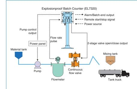
Combined with a flowmeter and valve, the batch counter measures a predetermined amount of process fluid in batching operations. As a piece of explosionproof equipment, the batch counter is suitable for outdoor applications.
