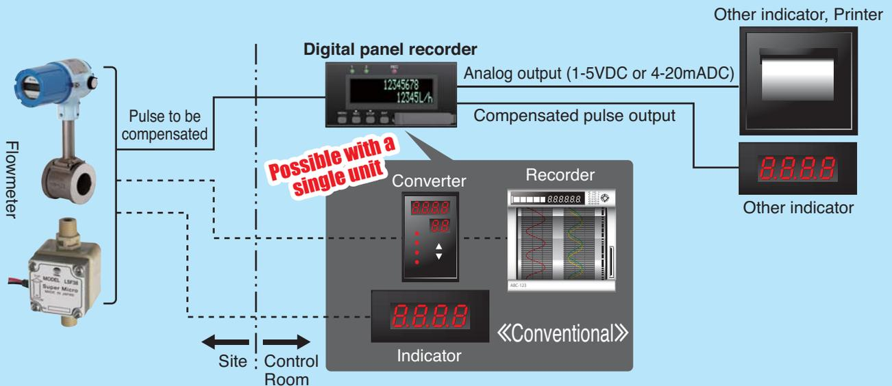
● **Pulse output and analog output functions are utilized for output to other indicator or the like.**
