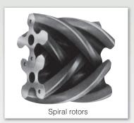
Each space formed by the rotors and the inner wall of the measuring chamber serves as a pocket (colored in blue) and, in one complete rotor revolution, the process fluid of eight times the volume of this pocket is delivered to the discharge outlet. Therefore, taking this rotor rotation by rotational frequency, we can measure the exact total volume of the process material delivered, while the instantaneous flowrate can be measured by the rotational velocity.
