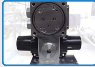
② Measuring unit (readily separable by taking off four screws.)
