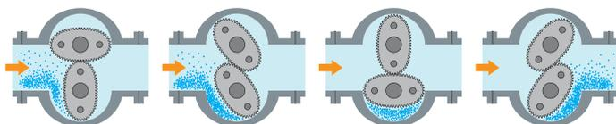
When the liquid flows, a pair of oval gears rotates, measuring a certain capacity (the part of crescent).
