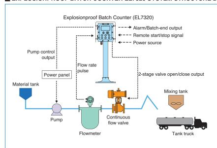
Combined with a flowmeter and valve, the batch counter measures a predetermined amount of process fluid in batching operations. As a piece of explosion proof equipment, the batch counter is suitable for outdoor applications.
